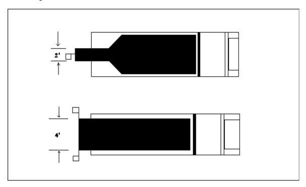
Warning Flags on Overlength Loads or Loads with a Rear End Overhang of More than Four Feet.
