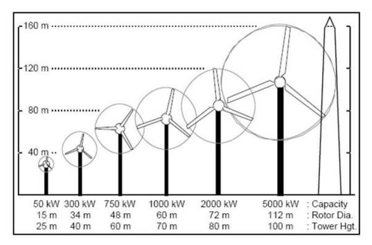
**Figure 8.18.** Schematic of wind turbine sizes (Connors and McGowan 2000).
